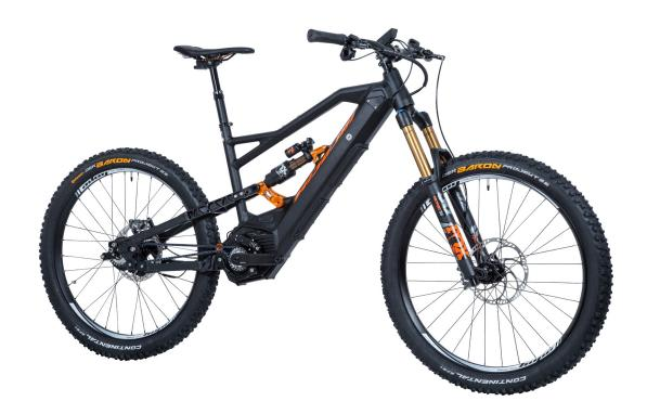
All GeoMetron models are built with short stems, so that the rider has a relaxed and comfortable seated position despite the long top tube.
