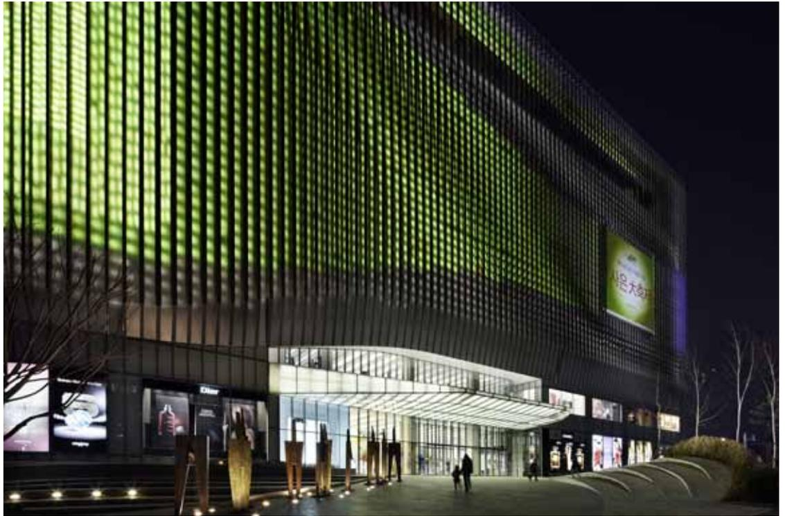
B2 | More than 22,000 LED spotlights are individually controlled by a DMX controller which coordinates them to produce unique façade lighting. Zumtobel realised the lighting solution project specifically in accordance with ag Licht's lighting design.
